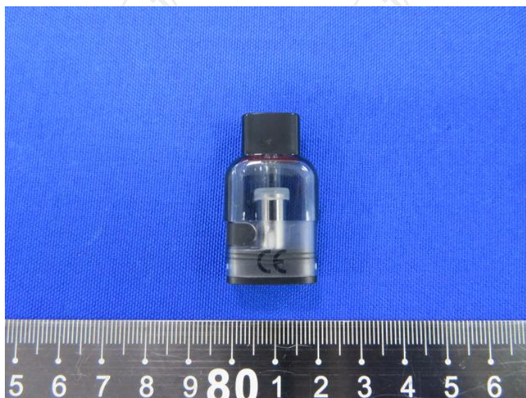
G GEEKVAPE K1 Cartridge 0.8Ω with 0.8ohm FeCrAl
